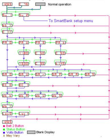
With a SmartBank Standard installed the SmartBank Setup menu (Su 2) will look like this:-
