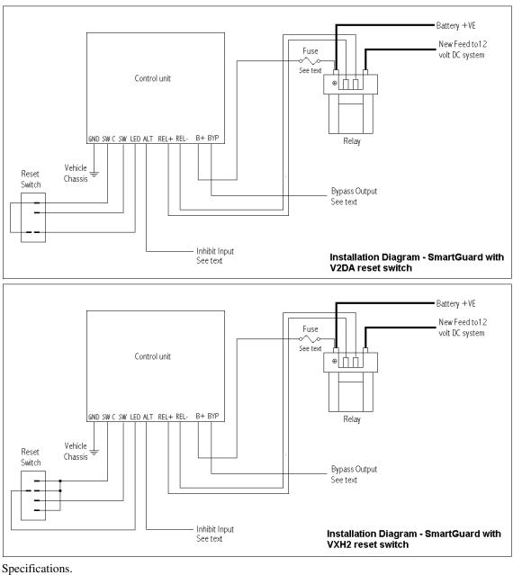
Specifications.Current consumption:-Standby< 0.2mA (< 200uA)</td>Relay actuation< 3 Amps</td>Shutdown< 12mA</td>Normal voltage operation range10 to 16 volts
